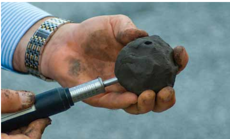
A pocket penetrometer is an example of a manual test that can be performed to determine soil type.
