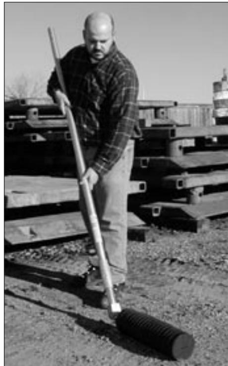
*If possible, always try to perform the work from outside the space. Michael Verner of TrenchSafety, demonstrates a Cherne remote placement plug designed for plugging lines in a sewer manhole from outside the space. Aluminum extension poles are available in lengths up to 24 feet.*
