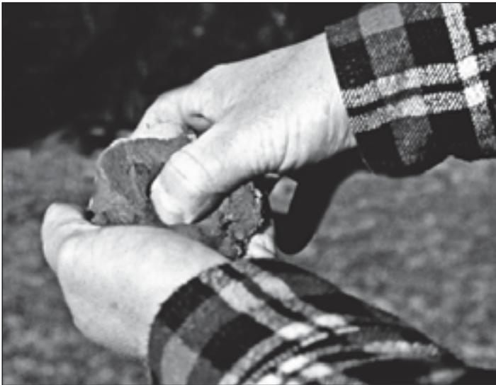
*The thump penetration test is the least accurate of all tests. However, it is an accepted method of determining approximate unconfined strength. Its accuracy relies on the experience of the person performing the test. Type A soils can be indented with difficulty. Type B soils can be indented with moderate effort. Type C soils can be penetrated easily, and can be molded with light finger pressure.*
