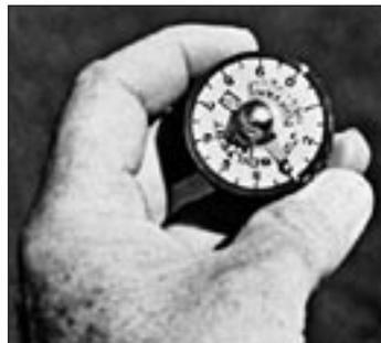
**A shear vane can be used to check the approximate unconfined compressive strength of cohesive soils.**
