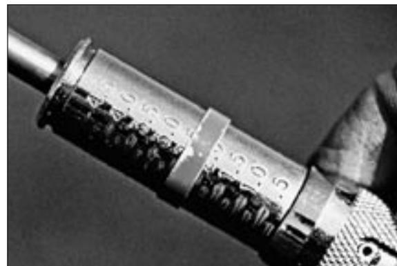
**A pocket penetrometer can be used in the field to check the approximate unconfined compressive strength of cohesive soils.**
