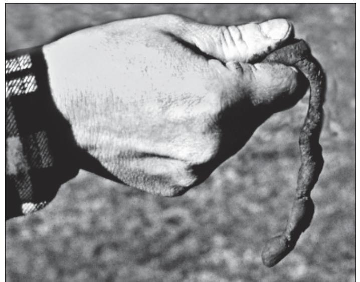
*The ribbon test is another test to determine whether a soil is cohesive or granular.*
