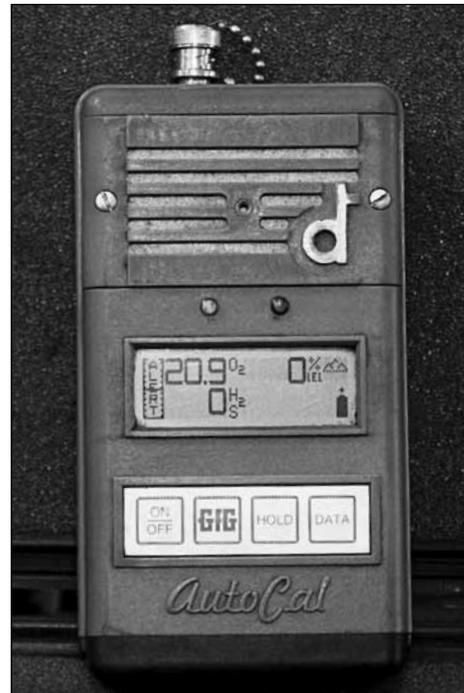
OSHA requires use of a direct-reading instrument for confined space work, meaning that the gas detector must display current readings in “real time.” This instrument indicates a normal level of oxygen (20.9%) and no other gases. Also, the battery is fully charged (bar graph in lower right corner of the display). The unit is operating in the peak-hold mode (mountain peak in upper right corner).
