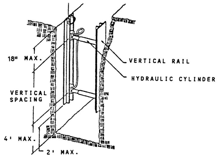
Figure 2. Pneumatic/hydraulic Shoring
